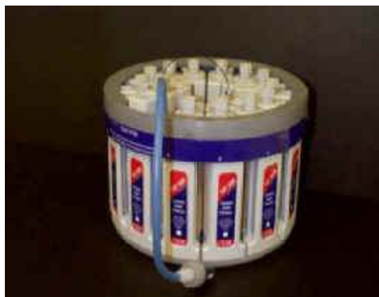
Figure 5. Carousel, showing pressure sensor and fiber optic temperature sensor attached to the control vessel and outer plastic ring around all of the support modules.
