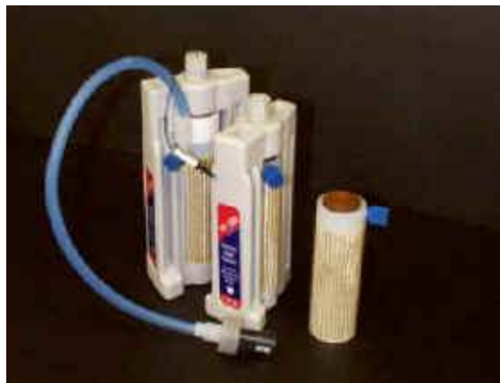
Figure 1. From left to right; control vessel in the support module with pressure sensor attached and fiber optic temperature sensor inserted, a typical reaction vessel in a support module, and an assembled reaction vessel showing the explosion-proof Kevlar sleeve and the load distributing cap piece placed on the vessel lid.
