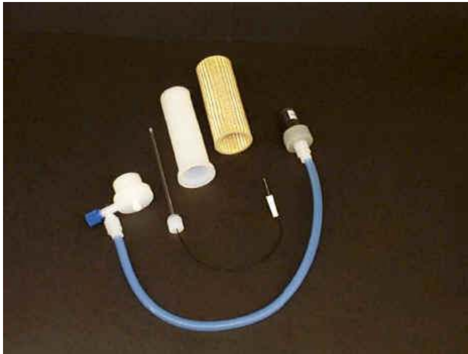
Figure 3. Control vessel parts, from left to right: Vessel lid with pressure release check valve and pressure transducer attached, glass thermal well with compression fitting and fiber optic temperature sensor, Teflon reaction vessel, Kevlar explosion proof sleeve, and pressure transducer.
