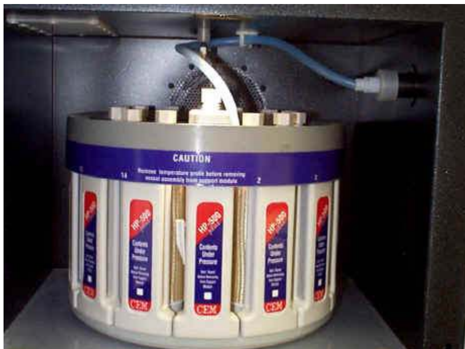
Figure 8. Inside the oven; showing the pressure and temperature sensor connections. The temperature sensor connection is located in the middle of the oven ceiling. The pressure tubing wraps around the temperature connector, and is attached to the oven ceiling with a removable plastic clip.
