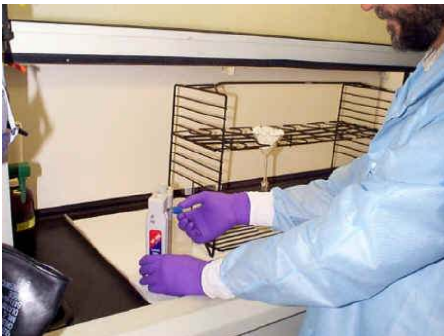
Figure 9. After the microwave digestion and the cool down period the pressure in the reaction vessels should be released by slowly unscrewing the blue cap and venting any remaining vapors in a fume hood.
