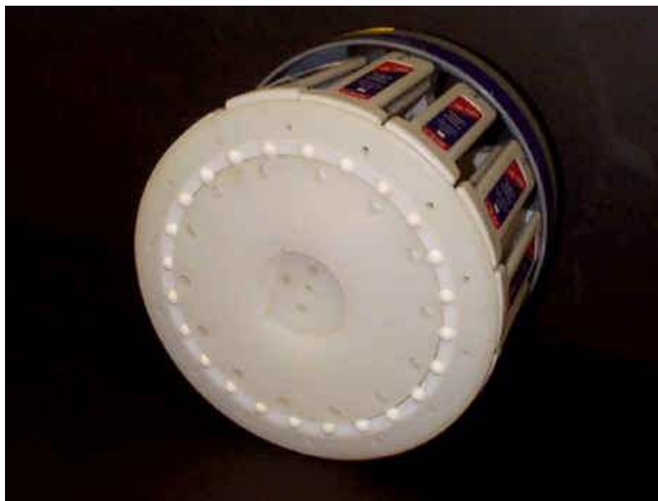
Figure 6. Carousel bottom; showing the ring of ball rollers and receptacle for the drive lug.
